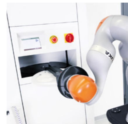
As a pre-setup operation, the LBR iiwa takes a component reel from the SIPLACE Tower.
