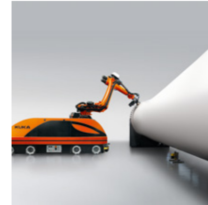
Mobile robotics for the precision machining of XXL components.
